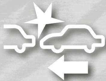
The system can be turned on or off by pressing the Forward Collision button on your touchscreen. You can also use your touchscreen to adjust the system's sensitivity and active braking status.
