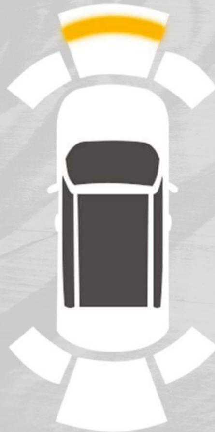
When the sensors detect an obstacle, a chime will sound and the ParkSense Park Assist warning will appear in the instrument cluster display. The system will show arcs in the area of the obstacle based on relative distance and location. As you approach the obstacle, the arcs will move and the chime will change from slow to fast to continuous.
